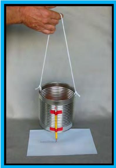
Tin can seismograph recording seismic waves.
